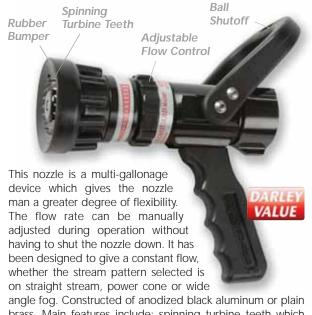
brass. Main features include: spinning turbine teeth which give excellent breakup of the water stream, flush mechanism, large ribbed rubber bumper, large rubber handle, dual Trunion drive on ball shut-off which provides smoother shut-off and less maintenance, ball shut-off is of the full flow type with chrome brass ball and nylon seats. Nozzle comes standard with 11/2" female NST. Ship. wt. 2-9 lbs. Adjustable to 30-60-95-125 gpm
