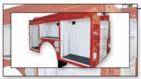
**BODY -** PolyBilt model 164 Integral Series Pumper-Rescue body with 1000 gallon integral tank. Limited lifetime body warranty is standard.
