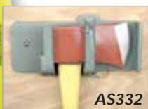
Designed for use with 6-pound flat or pick head axe. Bracket is 5"Hx2<sup>1</sup>/<sub>8</sub>"D. Expands from 7<sup>1</sup>/<sub>4</sub>" to 8<sup>1</sup>/<sub>4</sub>" W to fit most axe heads. 2<sup>1</sup>/<sub>2</sub>"Hx1<sup>1</sup>/<sub>4</sub>"W slot in end for pick to protrude. Axe blade protected by a replaceable plastic sleeve. Pinned handle holder accepts up to 2<sup>5</sup>/<sub>16</sub>"W handle. Stainless steel for trouble-free service. *Ship. wt. 4 lbs.*
