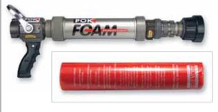
The Quick STIK system uses solid foam/wetting agent that is inserted into the specially perforated foam sleeve. Matched up with a 30-60-95-125 gpm adjustable nozzle, this Quick STIK system can deliver up to 600 gallons of foam/water mixture per stik.
