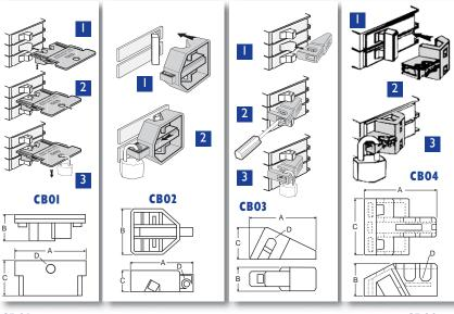
CB01 Our single pole breaker lockout requires a single toggle with a recessed hole in it.
