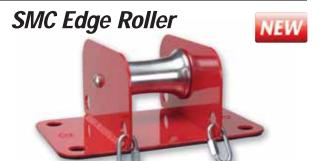
Reduce friction when going over the edge with the versatile RA/SMC Edge Roller. Two edge rollers connected by quick links will lay over a right angle such as a rack wall or edge of a building. This efficient 4" wide single edge roller ships with screw links for connecting two or more rollers together. Ship. wt. 5 lbs.
