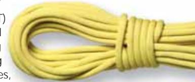
**RIT 900 6.8mm** - 100% aramid fiber search line. Designed with a supple hand to enable long lengths of cord to be stuffed in a pocket or bag, deployed efficiently, and easily tied with directional knots. Heat resistant to 932F.
