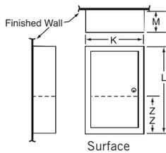
**Potter Roemer Detention Series Cabinets** provide the specifier with the substantial unitized design of 12 gauge cold-rolled steel construction for *maximum security* facilities. All corners are mitered and ground smooth to eliminate any dangerous projections. The heavy-duty continuous hinge adds to the secure features of these cabinets.
