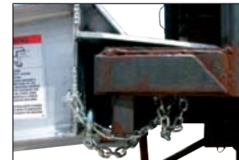
15" OVERLAP INTO TRAILER/BUILDING SAFETY CHAINS STANDARD
