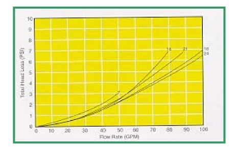
Initial Pressure Drop for ®Harmsco Cluster Filters in Clean Water. Water King Models HIF-7, HIF-14, HIF-16, HIF-21 and HIF-24.
