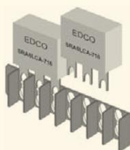
The Edco SRA6LCB slips under the equipment-side screws of the terminal strip. The protector ground wire must be bonded in a short, direct manner to the cabinet power ground. Protectors can be mounted consecutively along the terminal strip.
