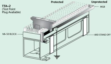
UNPROTECTED SIDE – TERMINATE FIELD SIDE WIRING COMING INTO BUILDING ON THE "UNPROTECTED SIDE"
