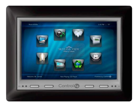
The Control4<sup>®</sup> 7" Wall-Mount Touch Screen is an intuitive way for guests and staff to manage room automation. Ideal for new construction and for existing properties, the 7" Touch Screen is easy to install and use, providing one-touch control of audio, video, temperature, lighting, drapes and services.
