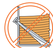
Nail too long
