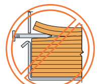
Nail at wrong angle
