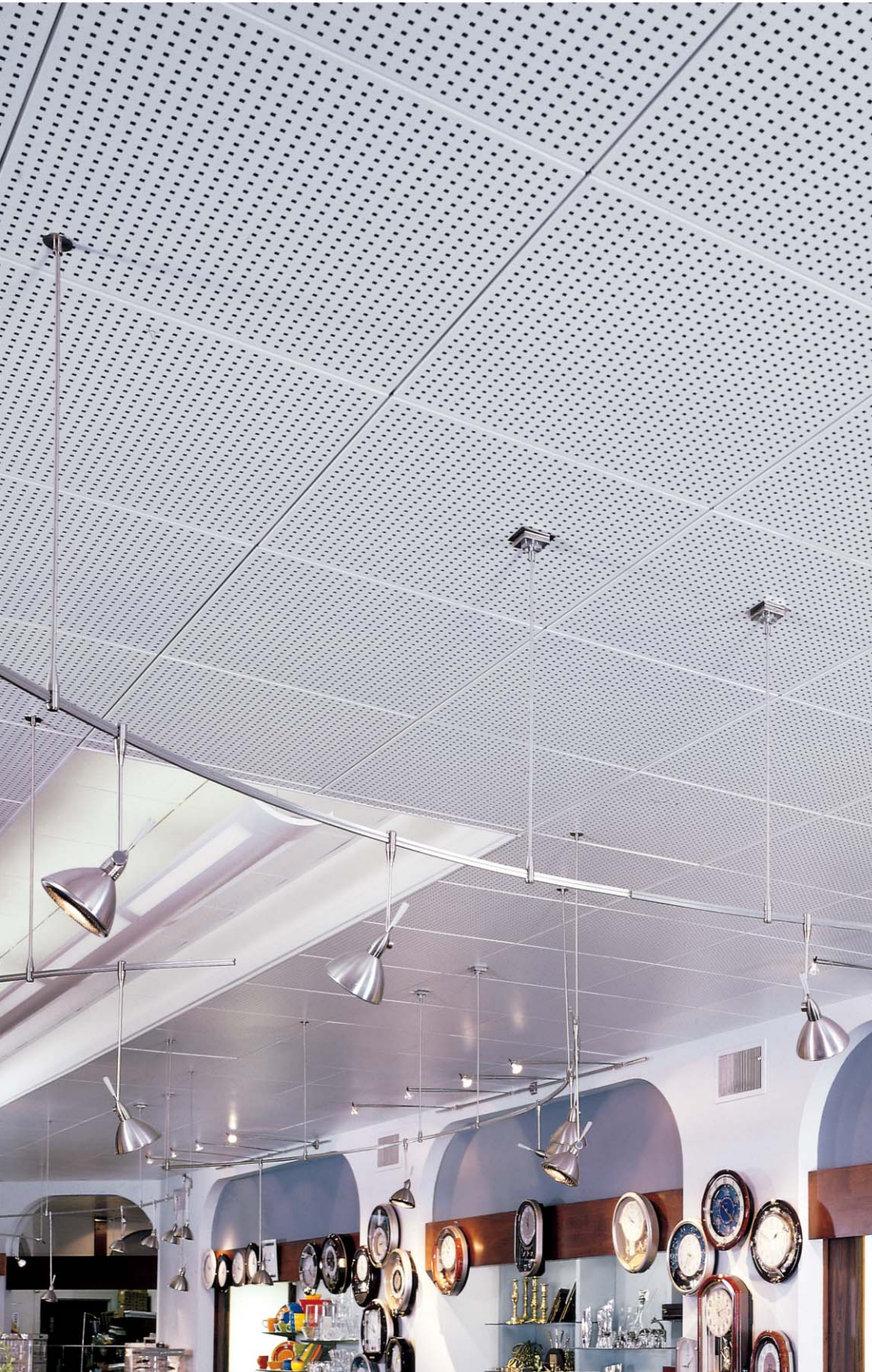
CELEBRATION Panel with D250 Perforation and Acoustical Backer, Installed Over Existing 2' x 4' 15/16" Suspension System and Acoustical Ceiling Panels
