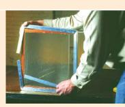
Seal the internal seams of the duct with silicon.
