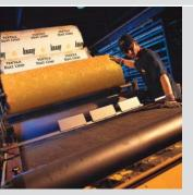
Knauf Textile Duct Liner is flexible, yet durable with a tough mat facing and an encapsulant edge coating to eliminate flaring.
