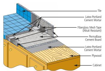
at least 3/8" and less than 5/8" from ends and edges. Ensure PermaBase is tight to framing.
