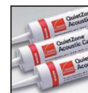
Acoustically engineered to block sound vibrations, QuietZone Acoustic Sealant is a silicone-enhanced acrylic mastic sealant that retains acoustic properties over time and won't harden for the lifetime of the product. It is used for gaps between wall stud plates and the subfloor; around electrical boxes, outlets, air ducts, doors and windows. The material is well suited for both interior and exterior caulking applications.
