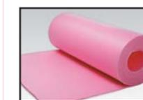
Made of lightweight, closed-cell polyethylene foam, QuietZone Acoustic Floor Mat is designed to isolate sound vibration and reduce impact noise. It is applied between the subfloor and a plywood or gypsum concrete overlayment that then "floats" on the mat. The material is lightweight and easy to cut and install.
