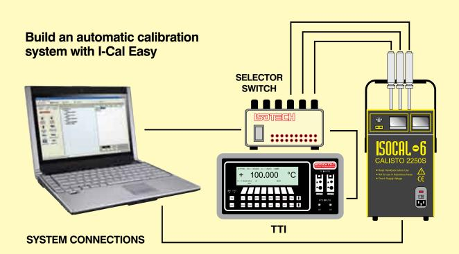
The number of sensors that can be calibrated depends upon the equipment used. Calibrate up to 16 sensors with two switch boxes, expandable to 32.
