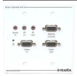
The Intelix DIGI-VGASD-WP-S active send balun distributes VGA video, stereo audio, and control signals over a single twisted pair cable, such as Cat 5 or Cat 6. The units mounts into a double-gang, double-deep wallbox and features a local monitor output.
