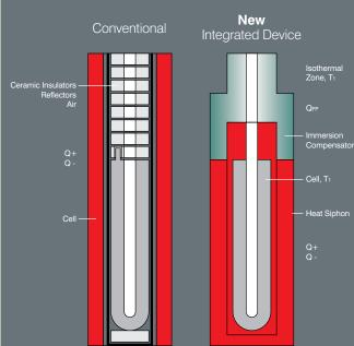
A fixed point cell is not long enough to eliminate heat conductance along the thermometer calibrated in it. Currently, using long furnaces, heat shunts and reflective baffles an attempt is made to reduce these losses.
