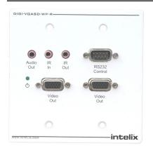
The Intelix DIGI-VGASD-WP-R active receive balun distributes VGA video, stereo audio, and control signals over a single twisted pair cable, such as Cat 5 or Cat 6. The unit mounts into a double-gang, double-deep wallbox and features dual amplified outputs and adjustable video equalization.
