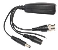
The Intelix S-V1CP transmits composite video, two conductor control, and power over a single twisted pair cable, such as Cat 5 or Cat 6. Used in pairs, S-V1CP baluns replace bulky coaxial video cable and utilize a building's existing structured cabling network.
