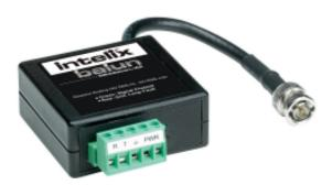
The Intelix V1-AR Active Receiver Balun allows the transmission of video signals up to 1 mile (1.6 km) via Cat 5 twisted pair cable when used in conjunction with a passive Intelix V1 or V1-ST video balun. The V1-AR features Automatic Gain Control (AGC) and Ground Loop Blocking (GLB) for reliable and stable image quality. Once installed, no adjustments to the V1-AR are needed.
