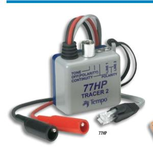
Permits technicians to identify the conductor within a bundle, at a cross-connect point or at the remote end. Can be used on twisted pair wiring (telecom, datacom, etc.), single conductors, coaxial cables, de-energized AC wiring and most other wiring.
