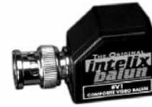
The V1 Video Balun eliminates 75-ohm coaxial cable and allows composite baseband video to be transmitted via single unshielded twisted pair (UTP) wiring in a Structured Cabling System. V1 Baluns are used in pairs to transmit standard NTSC, PAL, or SECAM composite video.
