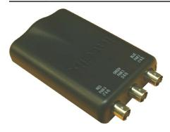
The Intelix AVO-V3 transmits one RGB signal or three composite video signals over structured cabling, such as Cat 5. Used in pairs, AVO-V3 baluns replace bulky RGB video cable and utilize a building's existing Cat 5/LAN cabling.
