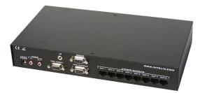
The Intelix DIGI-VGASD-T8 distribution balun sends a single VGA video and stereo audio source to eight remote destinations over inexpensive twisted pair cable. In addition, the unit extends RS232 or IR control signals over the same cable.
