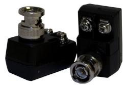
The Intelix S-V1ST transmits composite video over a single twisted pair cable, such as Cat 5 or Cat 6. The S-V1ST features a male BNC connector for direct connection to source and destination devices, as well as screw terminal connectors for quick twisted pair connection. Used in pairs, S-V1ST baluns replace bulky coaxial video cable and utilize a building's existing structured cabling network.
