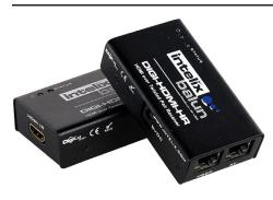
The Intelix DIGI-HDMI-HR transmits a highdefinition HDMI signal up to 150 feet over two inexpensive twisted pair cables, such as Cat 5e or Cat 6. The DIGI-HDMI-HR HDCP compliant supports 1080i high- definition video and is HDCP compliant. Each DIGI-HDMI-HR includes one send unit, one receive unit, one power supply, and two mounting brackets. The system is powered on either the send or the receive end. Power and status LEDs provide visual diagnostics.
