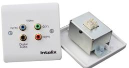
The Intelix AVO-V3AD-WP110-UK wallplate balun transmits one component video and one digital audio signal over standard unshielded twisted pair cabling. such as Cat 5 or Cat 6. Used in pairs or with a compatible Intelix balun, the AVO-V3AD-WP110-UK transmits signals up to 500 feet and is ideal for corporate A/V, churches, schools, auditoriums, and almost any other situation involving audio/video distribution.
