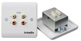
The Intelix AVO-A4-WP110-UK wallplate balun transmits four mono or two stereo analog audio signals over standard unshielded twisted pair cabling, such as Cat 5 or Cat 6. Used in pairs or with a compatible Intelix balun, the AVO-A4-WP110-UK transmits analog audio in either direction up to 2,500 feet and is ideal for corporate A/V, churches, schools, auditoriums, and almost any other situation involving audio distribution.
