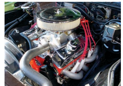
Insultherm Spark Plug Boot Sleeves can rest directly on hot headers and other engine components without burning, melting or becoming brittle.
