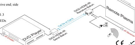
\* Distances may be affected by cable grade, cable quality, source and destination equipment, RF and electrical interference, and cable patches. Intelix specifications are based on straight-through cabling. www.intelix.com
