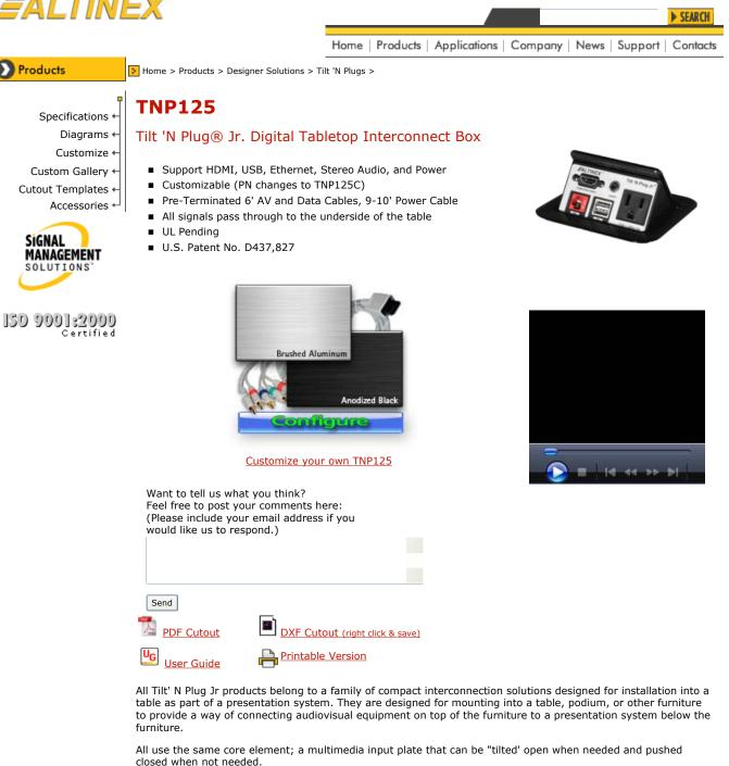
All signals pass through the input plate directly to cables on the underside of the table with no intervening circuitry. The use of additional ALTINEX Signal Management Solutions such as computer video interfaces, distribution amplifiers, and swithchers may be desirable.
