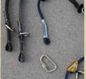
Remove body support carabiner on rope end and thread through D-ring on distribution strap.
