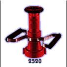
Combination fog nozzle. Moulded from polycarbonate with 2 1/2" attaching threads. Ideal for commercial and industrial hose installations. Available threads: NHT, NY Corp., NY(FD) Chicago (FD), CSA (5 X 3 1/8"), B.C. and A.M.A. (8 X 3), Nova Scotia Std. (5 X 3 1/4") Height - 5 1/4"; Gallonage - 150 GPM (US); ULC Listed
