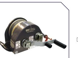
Universal Material Handling Winch w/ Removable Handle: The Universal Material Handling Winch includes a removable aluminum crank handle to utilize both our 9:1 and 4:1 drives. These two drives offer the capability of retrieval/descent at average speeds from 13ft/min (4 m/min) for loads over 50lbs up to 30 ft/min (9 m/min) for loads under 50 lbs.
