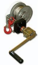
The *UCL Material Handling Basic Winch* offers a 500lbs-working load for material handling at 5:1 safety factor. The winch offers a removable handle with and a 3/16" x 70 foot galvanized cable assembly that comes with a heavy-duty forged material handling hook. Offered in Stainless Steel and Zinc Plated steel, not exactly as shown. Please call for your UCL representative for further details.
