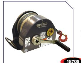
Universal Material Handling Winch w/ Permanent Mounted Handle: The Universal Material Handling Winch includes a permanently mounted handle to the 9:1 hub drive with an average speed of 13ft/min (4m/min). This handle offers durability, a foldaway handle and is simple to use.
