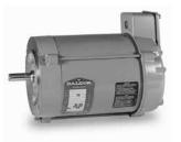
Features: Sealed fit at endplates. Sheds water. Conduit box cast into front endplate. Epoxy paint. High overload capabilities. The "P" indicates less pulley endplate for integral mounting; can be field modified for older designs with internal thru bolts. Operable at 50/60 Hz. 1.00 service factor.
