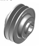
**Features:** Designed for up to 40 HP @ 1750 RPM. Used with A, B, 3V & 5V belts **Note:** DO NOT use these gray cast iron sheaves with rim speeds in excess of 6500 feet per minute.
