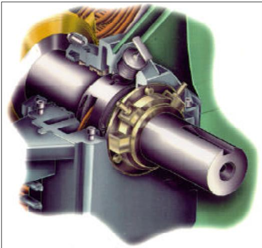
Since all sleeve bearing designs are allowed to float between geometric and magnetic centers, sleeve bearing motors need to be connected to their driven equipment with a limited end float coupling. USEM's sleeve bearings are provided with babbitted thrust face(s) to prevent damage that can occur if rotor is allowed to momentarily oscillate freely and bump the bearing. These babbitted bearing faces are not designed to provide for continuous axial thrust protection.
