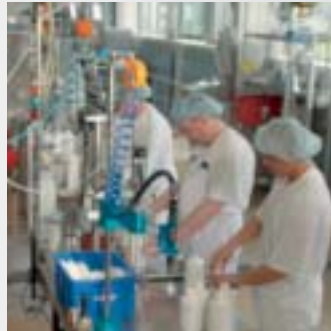
In filling processes, positive pressures must prevent the inflow from contaminated surrounding areas.
