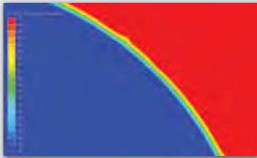
Thermal gradient as air passes through porous fabric
