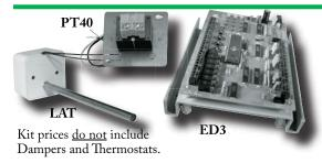
ED microprocessor zone control panels are suitable for all 2,3 and 4 zone applications. The panels are configurable and can be used for conventional heat-cool, heat pump, dual fuel heat pump, geothermal and even hydronic and oil systems. Kits include a 24 volt 40va transformer, a control panel, and a supply air temperature sensor. The ED4 is especially well suited for applications where building codes require fresh air intake.
