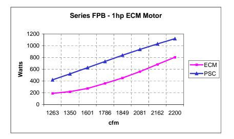
Another unit with ½ hp ECM motor kW is shown in comparison to a standard permanent split capacitor motor. The average watt reduction over the above range is 178 watts.
