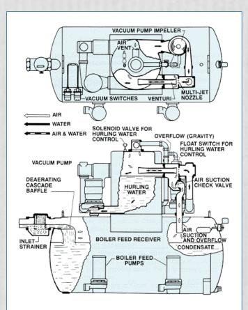
Series VCMD Style CMHD-A Cutaway Drawing
