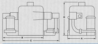
**STYLE CMHD-A** – air pump mounted as shown (dotted line) **STYLE CMHD-B** – air pump furnished separately
