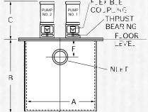
ALLOW B + C ABOVE FLOOR TO REMOVE PUMP & MOTOR ASSEMBLY
