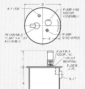
ALLOW B + C ABOVE FLOOR TO REMOVE PUMP & MOTOR ASSEMBLY
