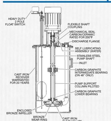
Note: TEFC and explosion proof motors are available. The motor horsepower requirement is often greater using explosion proof motors as they have unity service factor. A horsepower increase is not necessary using TEFC Motors.
