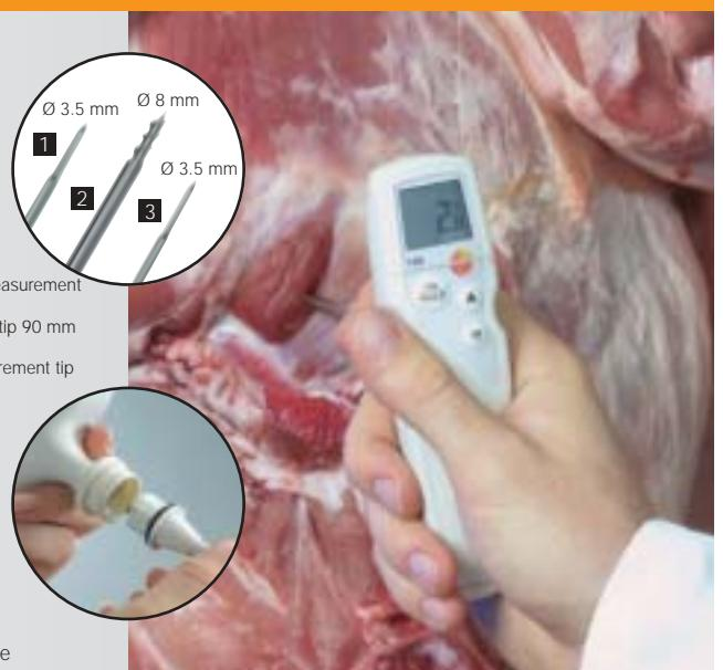
Penetration temperature measurement prior to further processing
