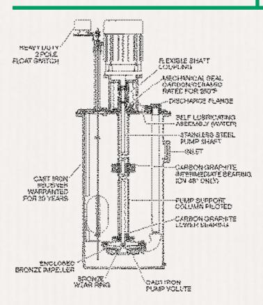
**Note:** TEFC and explosion proof motors are available. The motor horsepower requirement is often greater using explosion proof motors as they have unity service factor. A horsepower increase is not necessary using TEFC Motors.
